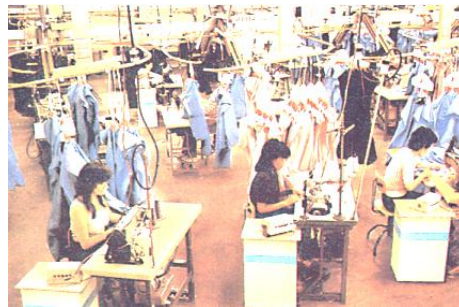
Fig. 1: Straight line system with hanger transport
